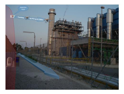
DFSL recommends using fixed HD cameras, whose total field of view covers the detector scanning sector, i.e. 100 degrees. The geometrical position of the HD cameras should be aligned with the Laser Curtain in order to provide a proper coverage. Please see the following illustration:
